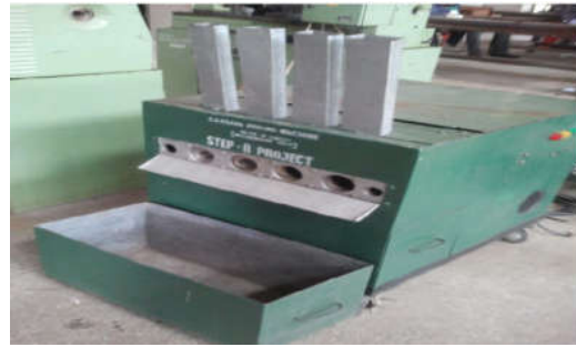
Fig. 20: A Model of the cassava peeler (Aniedi et al., 2012)
