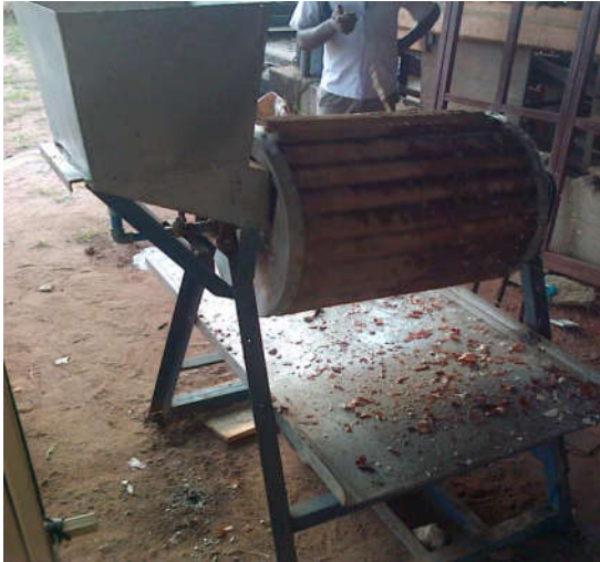
Fig. 33: The modified cassava peeler
